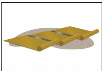
Fig. 1: VaporBlock® Plus™ Overlapping Roll-out Method
