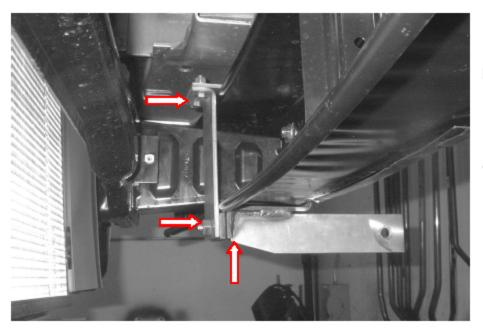
STEP 7. POSITION ONE OF THE 5038B SUPPORT BRACKETS BEHIND THE BUMPER AND ATTACH IT TO THE TOP OF THE MOUNTING BRACKET USING THE 3/8" X 1 1/4" BOLTS, WASHERS AND NUTS AND TO THE BOTTOM USING THE 1/2" X 11/2" BOLT, SPACER, WASHER AND NUT. (FINGER TIGHTEN ONLY!)
